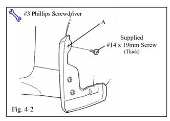
(b) Install supplied #14 x 19mm (thick) screw in location A while holding part up and into body panel then tighten. Do not overtighten (Fig. 4-2).
